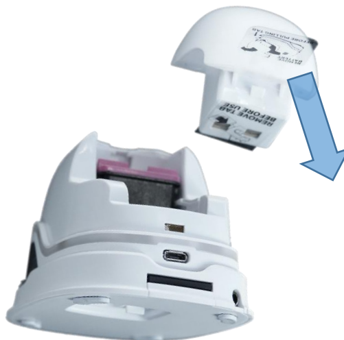
Fig. 9: Battery contact insulating tape
