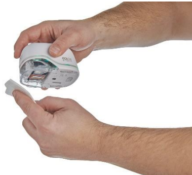
Fig. 28: Clean print head with damp cloth
