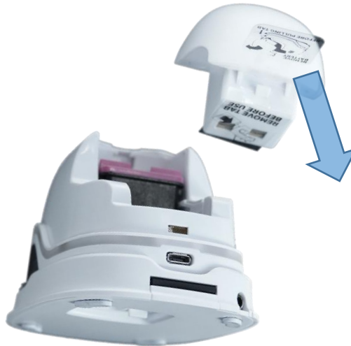
Fig. 9: Battery contact insulating tape
